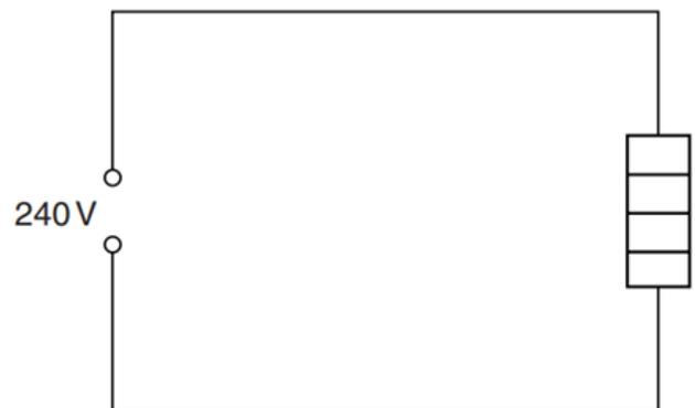
The wires used to connect the heater to the power supply each have length 75 m. The wires have a cross-sectional area 2.5 mm<sup>2</sup> and resistivity 18 n $\Omega$  m. The heater has a constant resistance of 38  $\Omega$ .
