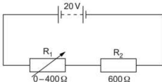
The resistance of  $R_2$  is 600  $\Omega$ . The resistance of  $R_1$  is varied from 0 to 400  $\Omega$ .
