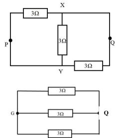
So the equivalent circuit is simply three,  $3\Omega$  resistors in parallel, so the equivalent resistance is  $1\Omega$ .
